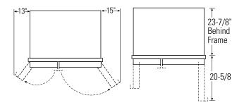
Allow minimum clearances for freezer door and fresh food door for a full 130° door swing and to allow for pan removal.
